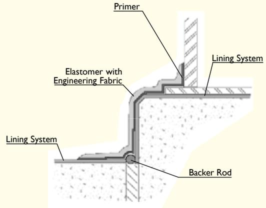
Seal for Tank Bottom and Foundation Treatment
